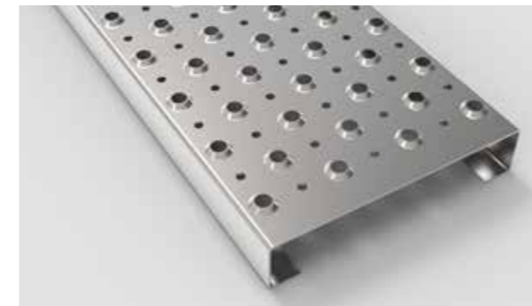
Type AP 2 - 50 with drainage (MAW) Type AP 3 - 50 with drainage (MAW) Anti-slip perforation \varnothing 14 mm punched up 4 mm high. Drainage perforation flat \varnothing 8 mm both on a 50 mm c.t.c staggered pitch.
