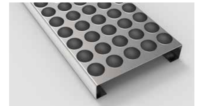
Type AP 2 - 50 rubber caps (DOP) Type AP 3 - 50 rubber caps (DOP) Perforation \varnothing 14 mm, c.t.c. 50 mm, 4 mm deep, also with drainage perforation \varnothing 8 mm if required, c.t.c. 50 mm, 0 mm deep. Suitable for using rubber caps. Preferred widths in multiples of 50 mm.
